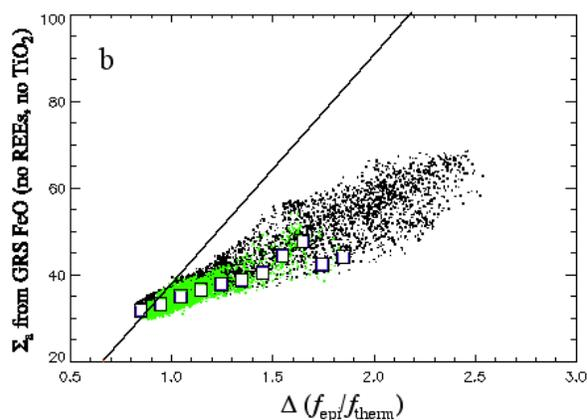
Fig. 1. Partial macroscopic absorption cross section vs. epithermal to thermal flux ratio.
