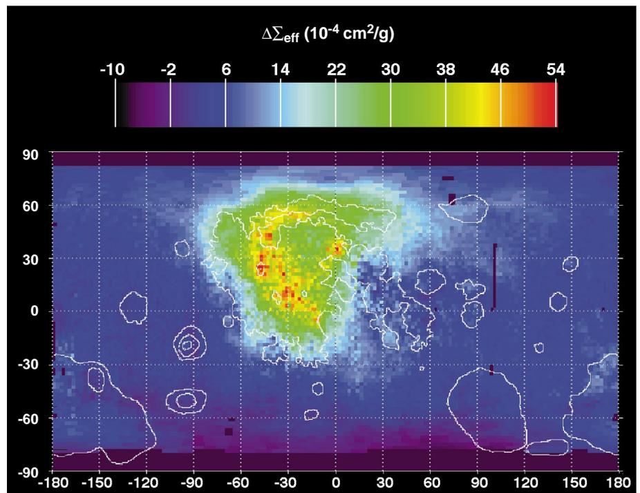
**Fig. 4.** Map of  $\Delta\Sigma_{\text{eff}}$ , a measure of thermal neutron absorbers in addition to Fe, Ti, and other major elements implied by CSR-derived abundances. The greatest values of  $\Delta\Sigma_{\text{eff}}$  are found surrounding the Imbrium basin, approximately collocated with regions rich in KREEP.
